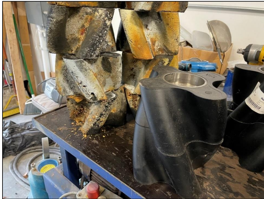
Damaged Vogelsang Rotary Lobes Compared to New Rotary Lobes
