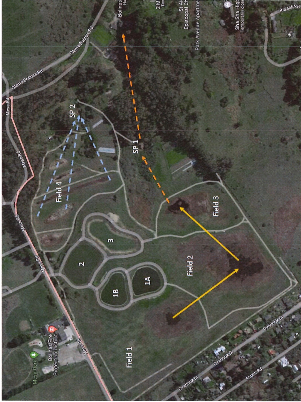
Figure 1. Bolinas Community Public Utility District Treatment Facility: Treatment ponds are labeled 1A and 1B, storage ponds are labeled 2 and 3, seepage ponds are labeled SP1 and SP2, and disposal spray fields are labeled Fields 1-3 (Field 4 is unused). Solid yellow arrows show wastewater flow between fields, dashed orange arrows represent overland flow to SP1 and off-site, and dashed blue arrows represent stormwater overland flow to SP2.
