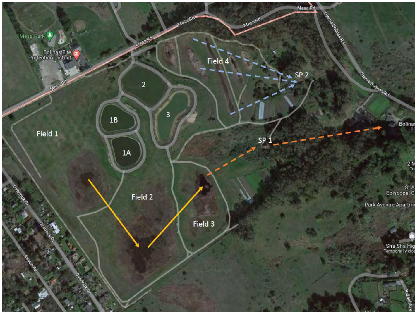
Figure 1. Bolinas Community Public Utility District Treatment Facility: Treatment ponds are labeled 1A and 1B, storage ponds are labeled 2 and 3, seepage ponds are labeled SP1 and SP2, and disposal spray fields are labeled Fields 1-3 (Field 4 is unused). Solid yellow arrows show wastewater flow between fields, dashed orange arrows represent overland flow to SP1 and off-site, and dashed blue arrows represent stormwater overland flow to SP2.
